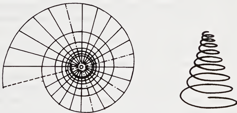
Figure 10-1. A hyperbolic spiral is characterized by its constantly changing curvature, inwardly concentrating as it moves towards the centre.
